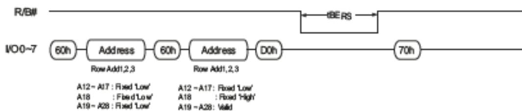
Figure 28: Multiplane Block Erase Operation
